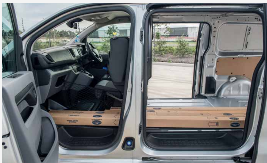
Load volume varies from 5.3m 3 to 6.1m 3 on the longer body, while load length is 2,512mm/2,862mm for the standard/long variants respectively.
